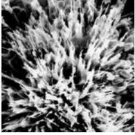
Slag and fly ash blended cement samples were treated with Xypex Admix and examined for evidence of crystalline growth at ages ranging from 8 months to 2 years. Samples were sliced and/or split and examined at magnifications between 500x and 5000x. Characteristic Xypex crystalline growth was observable on all Xypex treated samples, providing evidence of Xypex crystalline reactions with fly ash and slag blended cements.
