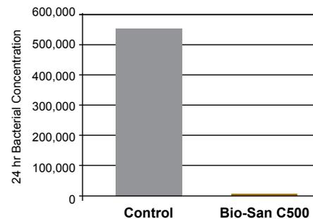
Concrete was cast in 100 x 200 mm cylinders with both control and treated mixes. A wastewater facility was chosen that had elevated  $H_2S$  levels and substantial existing MIC corrosion damage. Test samples were suspended in the air space of the tank for 10 years. Exposure trials showed that treated concrete had nine times less concrete mass loss compared to control samples.
