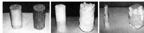
Xypex-treated mortar and untreated mortar were measured for acid resistance after exposure to a 5% H<sub>2</sub>SO<sub>4</sub> solution for 100 days. Xypex suppressed concrete erosion to 1/8 of the reference samples.
