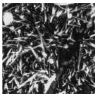
A 60 cm x 70 cm x 40 cm concrete block was cast and a Concentrate coating was applied to the surface and cured. The block was left outdoors for approximately 1 year. Subsequently, a 40 cm (15.75 in.) long cylinder was then cored perpendicular to the Xypex
